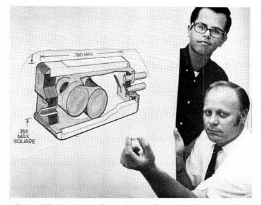
ENLARGED DRAWING shows detail of a tiny rolamite acceleration-sensing switch. The "force-bias" feature of the band holds the rollers in place until a pre-determined acceleration force causes the rollers to move, operating the switch. Fred Duimstra (2321), rolamite project group leader, holds the switch while Doug Schuler (2321), rolamite design engineer, displays the drawing.
